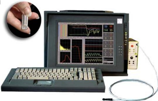
The targeted depth of sampling was specified by the spacing of the sending light source and the receiving light detector (Fig.2)
