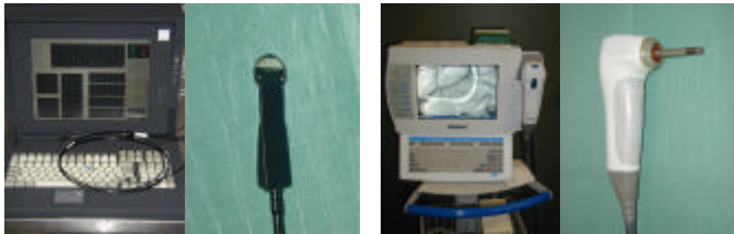
Fig. 1: (left) Oxygen2see device with combined NILDF/RS probe, (right) Cytoscan device with probe
